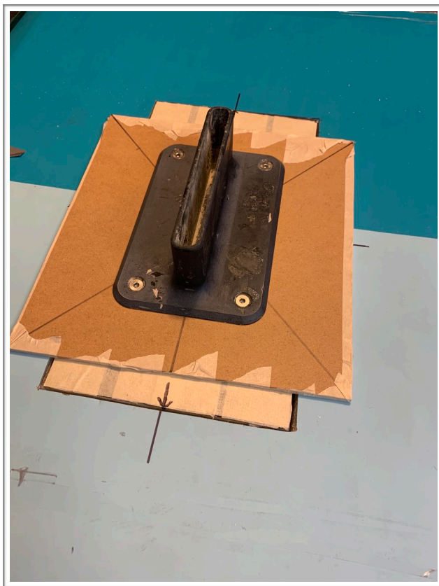
Figure 6 - Foil install aligned to crosshairs
